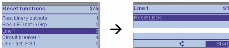
Figure 8-12 Reset Functions on the On-Site Operation Panel (for Example, Line FG)
